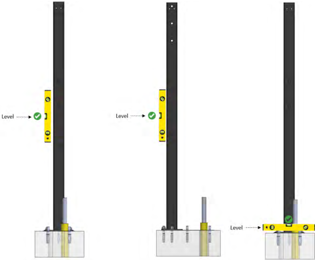
Fig. 43 - Checking pedestal base for level
