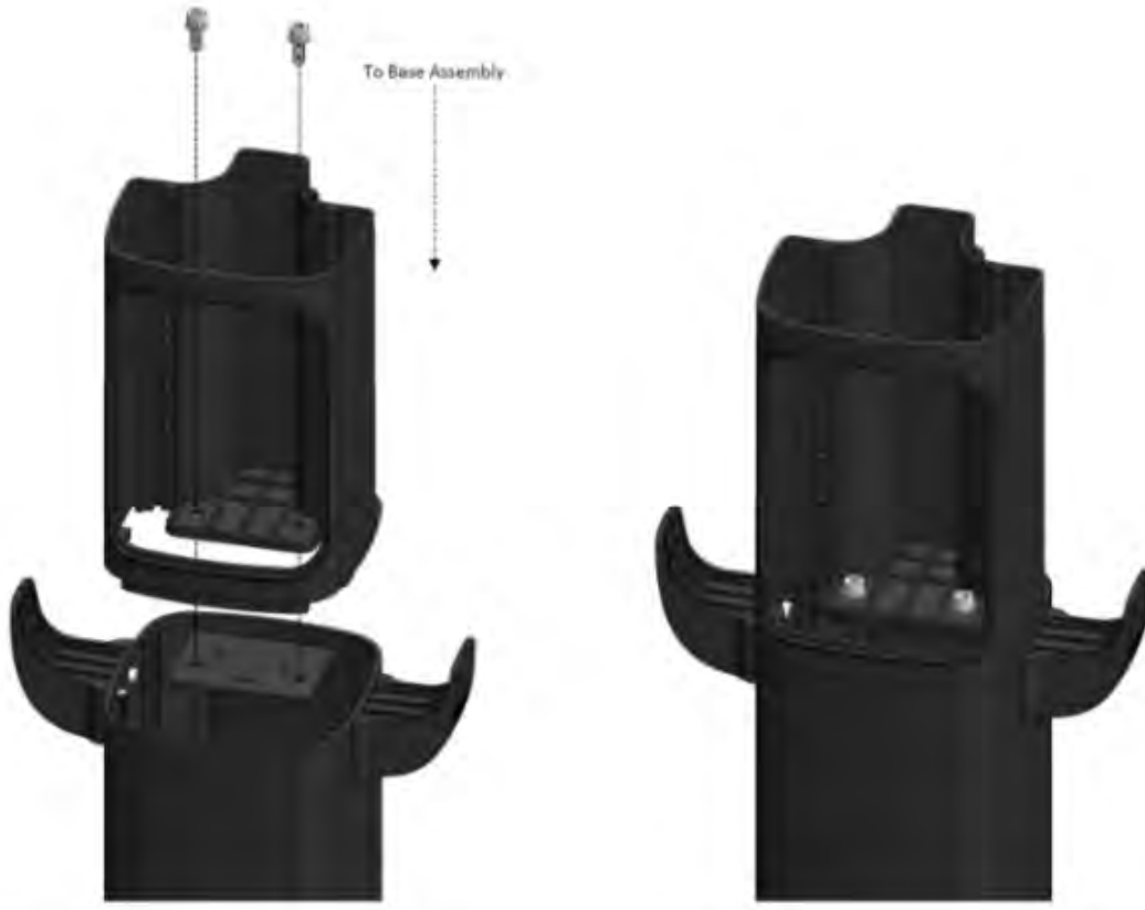
Fig. 22 – Installing pedestal top enclosure to base assembly
