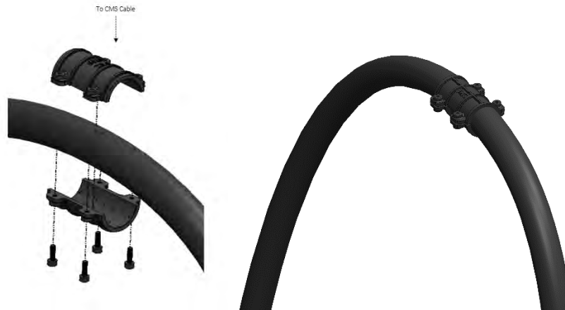
Fig. 53 – Installing CMS cable clamp
