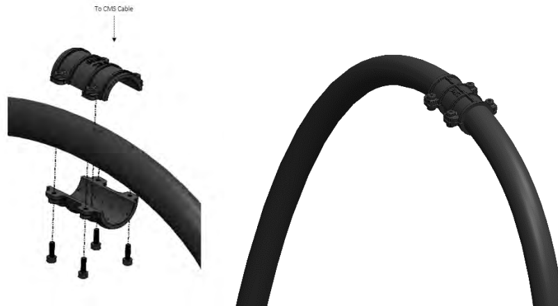
Fig. 46 – Installing CMS cable clamp
