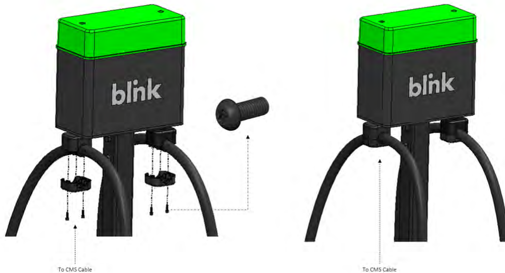
Fig. 47 – Installing CMS cable bottom and top cap
