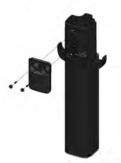
Fig. 14 – Remove Dual Holster Access Panel (2x T30 Tamper-Resistant Torx screws)
