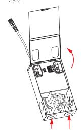
5. Insert the electrical supply cable through the KO; use appropriate bushing to prevent wire abrasion. Wire driver box (see *Wiring Diagram* on page 3 and illustration below).\*
