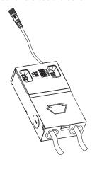
7. Insert driver box into ceiling in accordance with local/ national codes and connect the male and female connectors. Screw threaded nut over connectors to secure.
