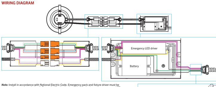
Note: Install in accordance with National Electric Code. Emergency pack and fixture driver must be on the same branch circuit. Ensure hot/live lead going to the black wire on the emergency LED driver is unswitched. When used with switched fixtures, the emergency pack must be wired ahead of the switch.
