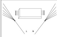
**6.** Insert Keystone Sign Hero LED tubes and rotate to desired position for optimal illumination. Ensure side marked "L" is connected to corresponding line socket and "N" is connected to corresponding neutral socket.
