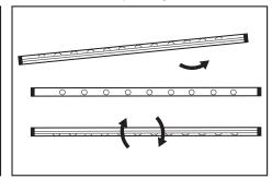
**7.** Place retrofit warning label on existing ballast (if applicable) or somewhere in sign. Ensure it is visible for all future maintenance. Close sign and apply power.
