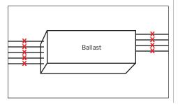
From mains, connect input (L) line to all wires coming from sockets on one side of sign and (N) neutral to all wires coming from the sockets on opposite end of the sign.
