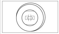
4. Access sign raceway/wiring box, and cut all ballast input and output wires as shown. Do not remove ballast if removal leaves an opening in the raceway.
