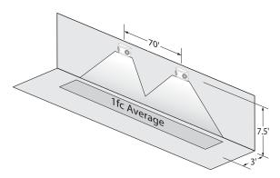
Using multiple NFT units (2.7W lamps) mounted at a typical 7.5' height delivers 63' on-center spacing with a 6' wide path of egress.
