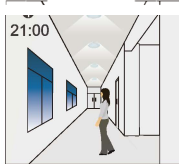
21:00 The light switches on at 100% when there is movement detected.
