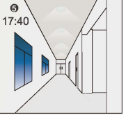
⑤ The light automatically turns on at 10% when natural light is insufficient (no motion).
