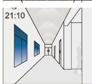
21:10 The light dims to stand-by level after the hold-time.
