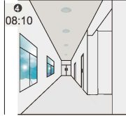
④ When the natural light level exceeds setpoint off to light, the light will turn off even if when the space is occupied.
