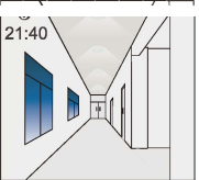
21:40 The light remains in dimming level at night.
